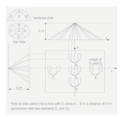
Disadvantage of the PIR technology is the need of the Fresnel lens, the ability to detect only remarkable human motion in tangential direction.
