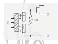
As the construction regards, PIR detectors incorporate a Fresnel lens in order to focus the radiation to the sensor elements, and also having dual or quadelements to subscract the ambient temperature and reduce the number of false alarms. PIR sensors can detect correctly horizontal movements, while radial movements cannot always be detected.
