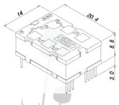
NJR4265 J1 is intelligent motion sensor that is designed for the sensing of short distance low speed movement object of e.g. pedestrian. The steady sensing of moving object is realized by embedded software. It is suitable for the built-in use of the sensing function to various equipments as all functions are
