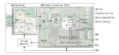
One of them is the NJR4265 from New Japan Radio Corporation, where antenna, RF circuit, IF amp, MCU and voltage regulator are integrated in a small package of the size 14 x 20.4 x 8.8 mm.
